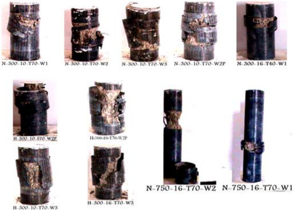
Figure ( 23 ) View of Failure pattern and fracture of some specimens
